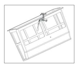
4.4.3 Re-install the filters, pay attention to the good position and slide the two clips to close the top cover.
